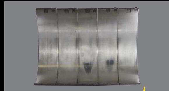
Connecting rod bearings and main rod bearings showed only normal wear, (as seen in the lower main bearings above) after 1.123 million km.
