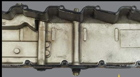
State-of-the-art lubricant technology promotes long oil life, evidenced by the valve cover, which stayed completely clean and free of deposits.
