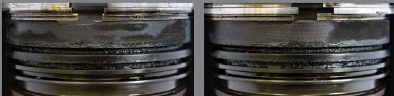
Pistons and piston rings exhibit no abnormal deposits and remain in good condition after more than a million km of service and oil drain intervals averaging 100,000 km.
