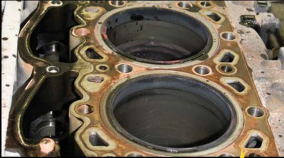
Original cross-hatching of cylinder walls are clearly visible, confirming that a potent film of protection was retained in the hottest part of the engine.
